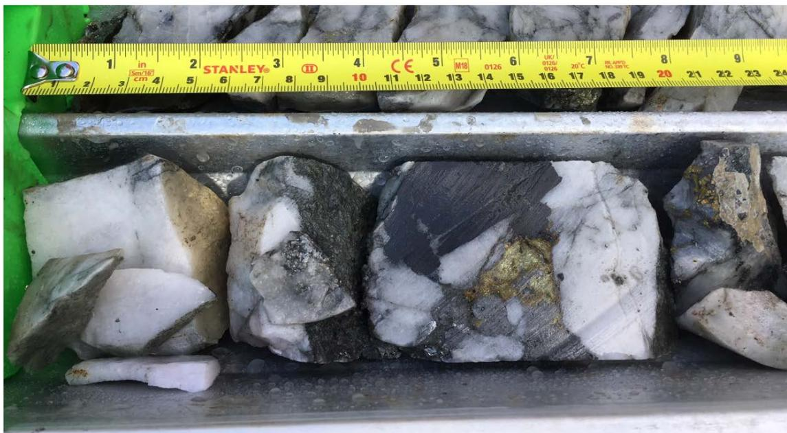
*Coarse wolframite in SVS quartz vein, drillhole CRD022, 410.70 m*
