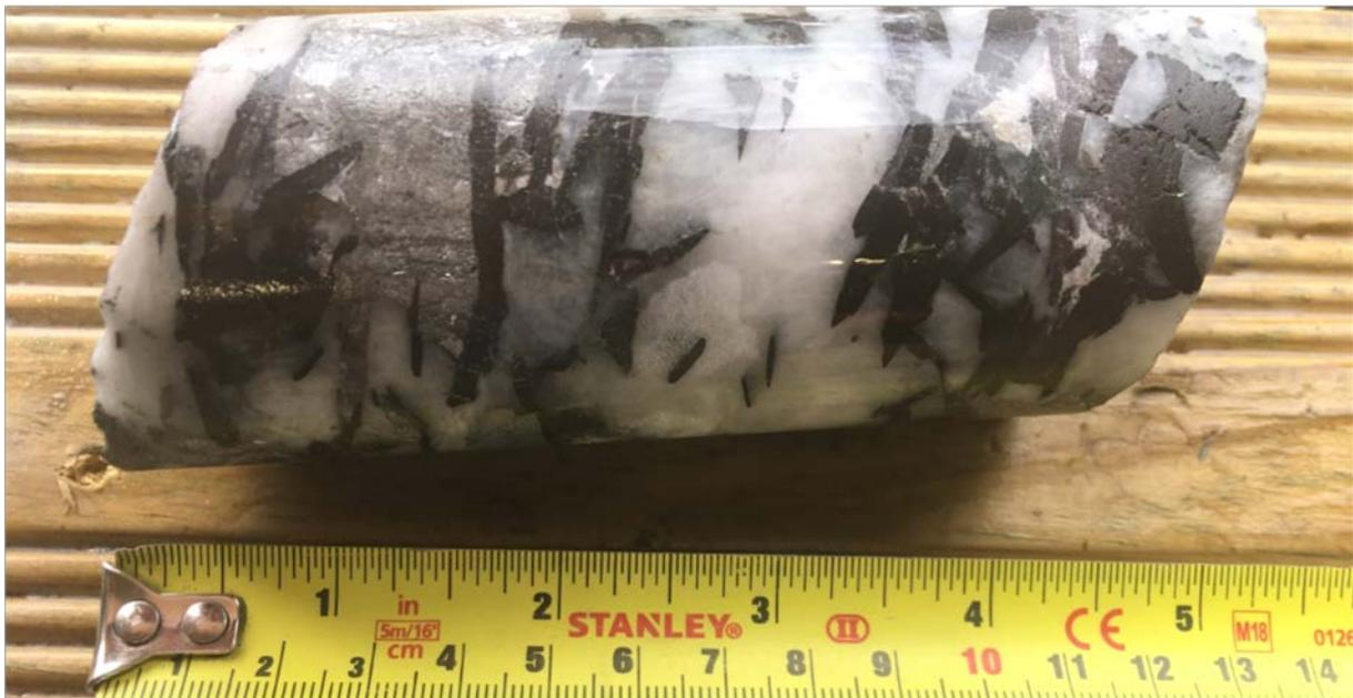
*Well-developed wolframite in SVS quartz vein, drillhole CRD021, 645.08 m*
