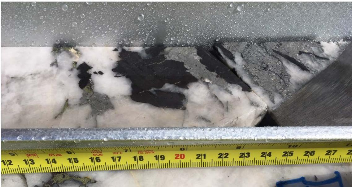
*Wolframite in SVS quartz vein, drillhole CRD022, 432.40 m*
