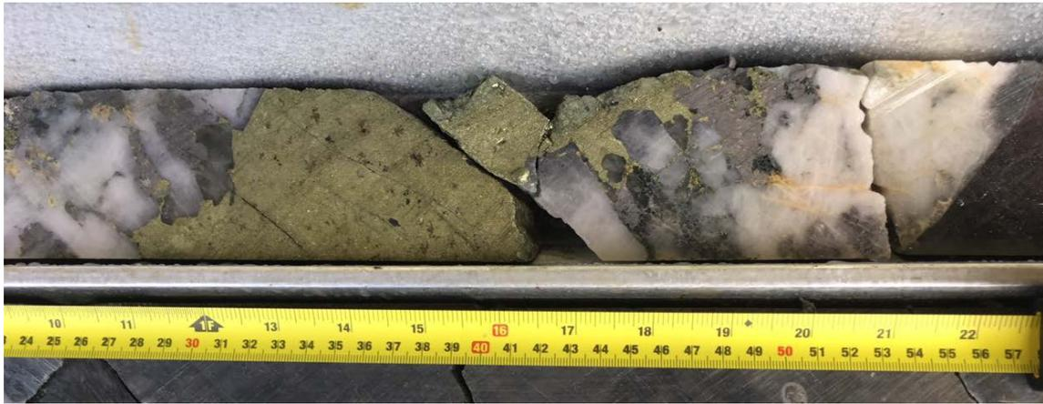
*Chalcopyrite-rich vein, drillhole CRD022, 449.31 m*
