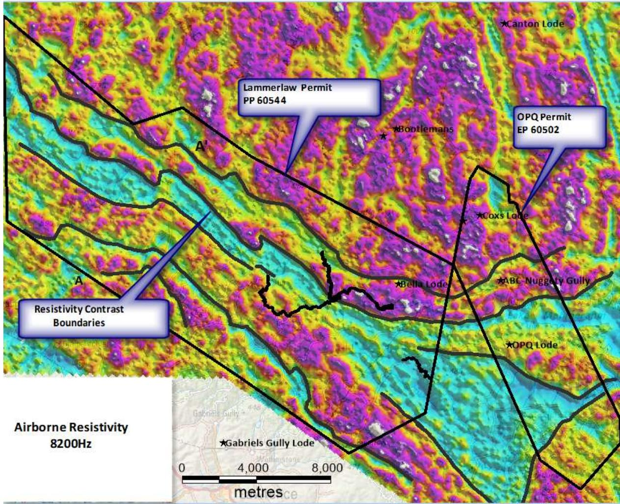
Figure 2 - Target areas on airborne resistivity
